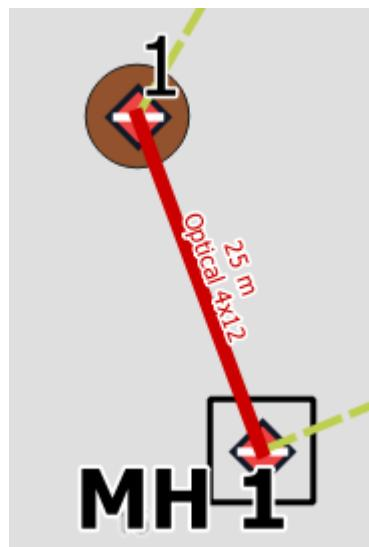
After you select **two elements** on the map and choose the cable laying option (route type + cable class), FiberQ opens the **Cable Parameters** dialog. In this dialog you enter and confirm all metadata for the new cable segment—such as **route type** (Underground/Aerial), **cable class** (Backbone/Distribution/Drop), **fiber type** (e.g., SM), **color code standard**, **number of tubes and fibers**, and additional technical fields (attenuation, dispersion, installation year, condition, etc.).
